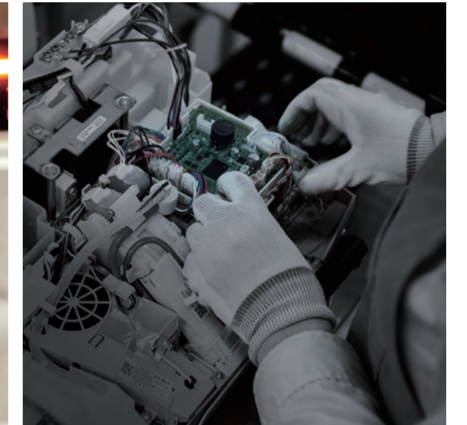
Assembling a shower toilet. In order to maintain accuracy and speed, INAX uses robotics technology in addition to the eyes and hands of skilled technicians.
